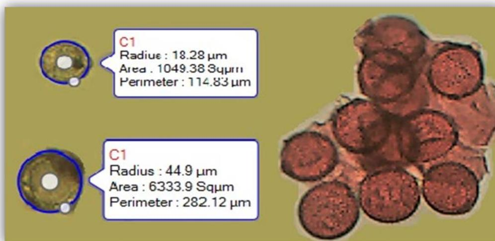
**Figure 15.** Microscopic view of pollen grains and their measurements.
