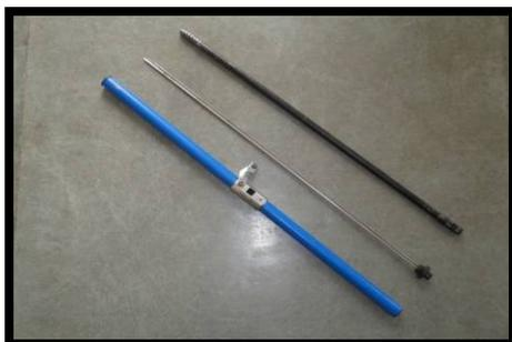
**Fig 3. Increment borer and its parts**
