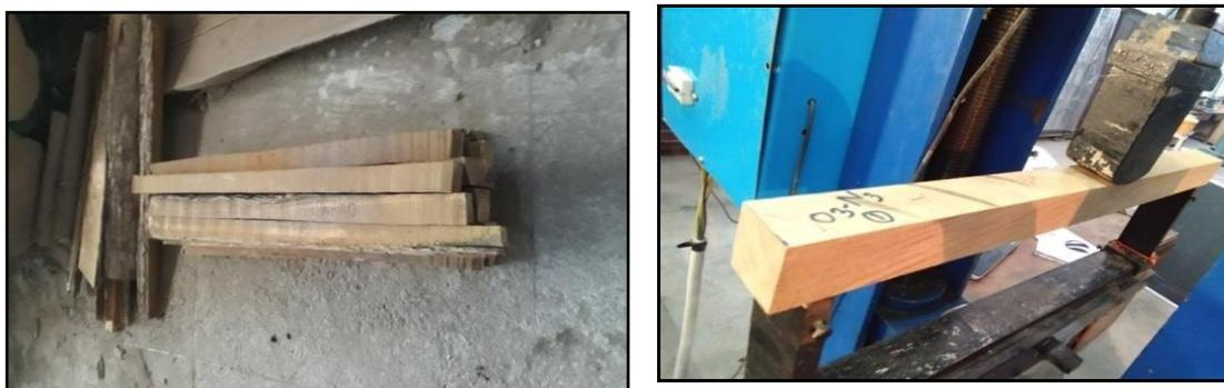
**Figure 14.a)** Preparation of samples from wood logs, and b) Testing of mechanical properties.
